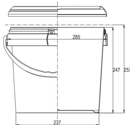
Measurements in millimetres
